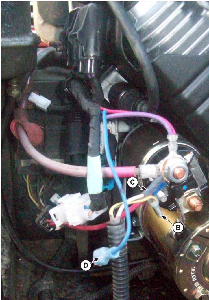
Figure 4. Connecting Lead Wires to Starter on Kohler EFI Engine.
